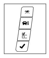
The buttons are the trip/fuel, vehicle information, customization, and set/reset buttons. The button functions are detailed in the following pages.
